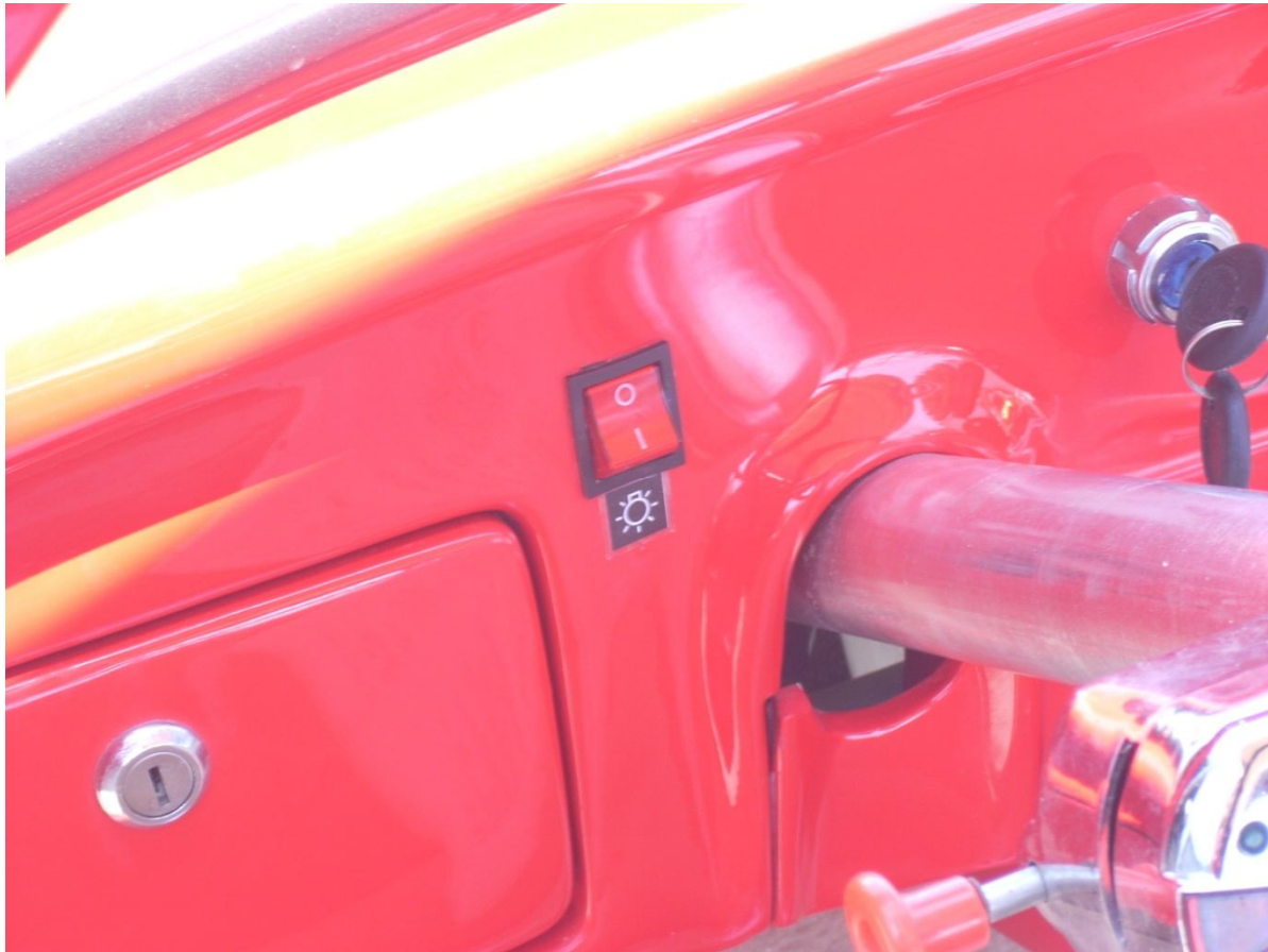
(Light switch shown in "OFF" position)
