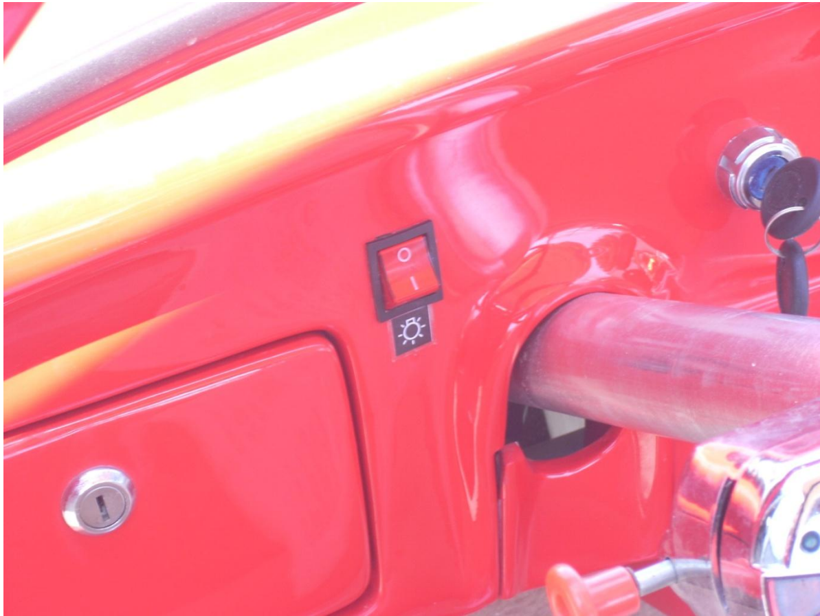
(Light switch shown in "OFF" position)
